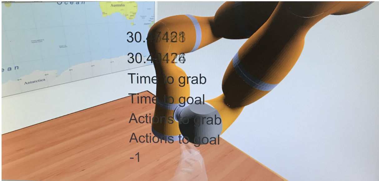
Figure 7.1: Kuka robot arm alongside transparent avatar used to aid the user in controlling the movement of the Kuka robot
